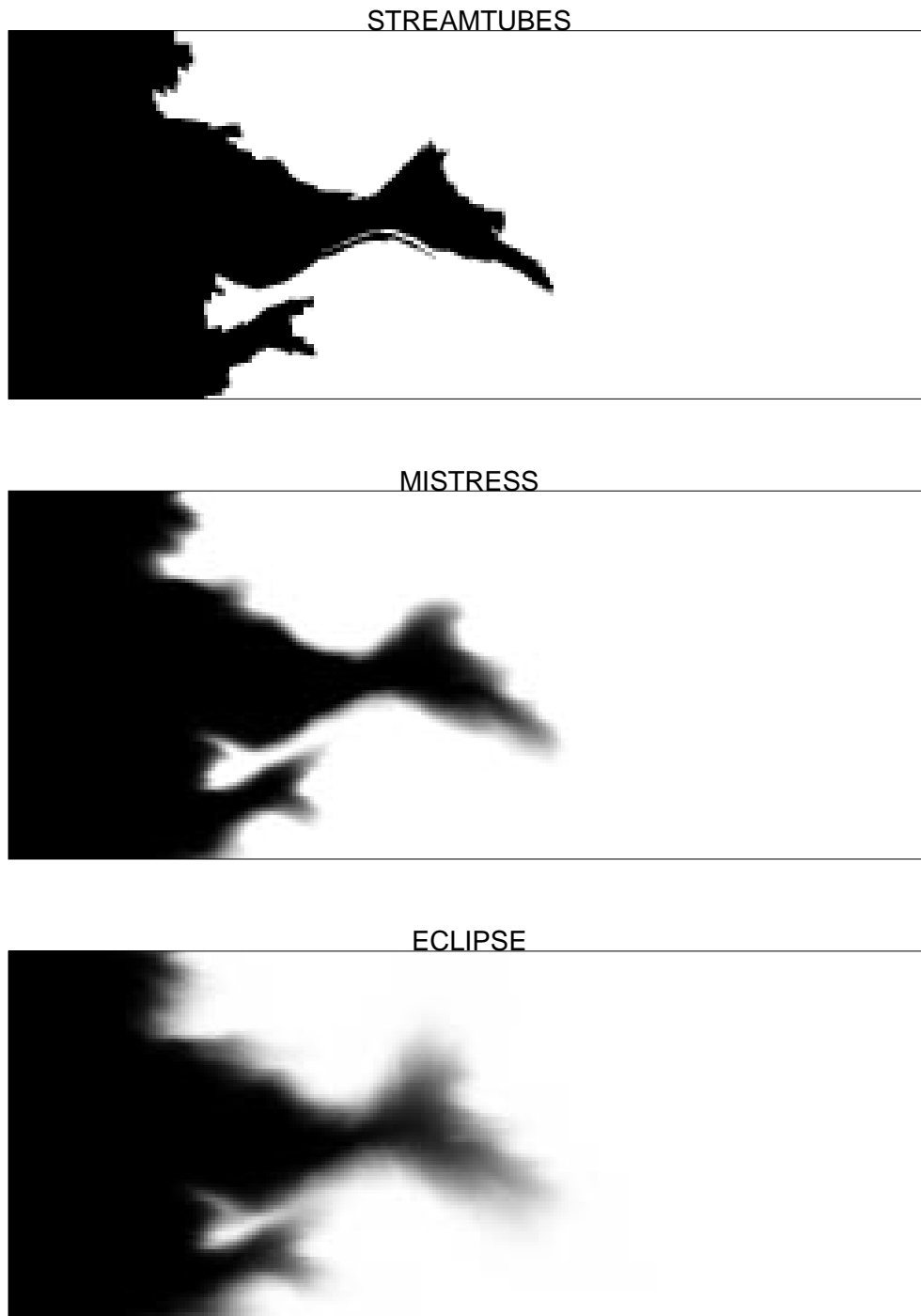
Figure 4.9: Comparison of concentration profiles showing the extent of numerical diffusion in finite difference simulators. Streamtube method versus Mistress, a research code with flux corrected transport (FCT) and Eclipse, a commercially available reservoir simulator with single point upstream weighting and automatic time step selection.
