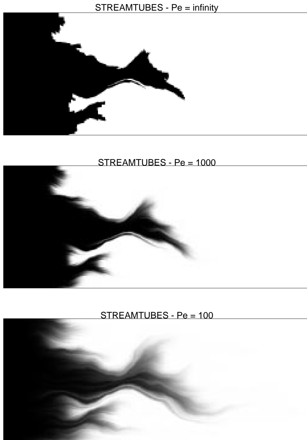
Figure 4.8: Including physical diffusion in M=1 displacement by mapping the convection-diffusion equation along each streamtube at t_D = 0.3 . Examples at N_{Pe} \rightarrow \infty , N_{Pe} = 1000 , and N_{Pe} = 100 .
